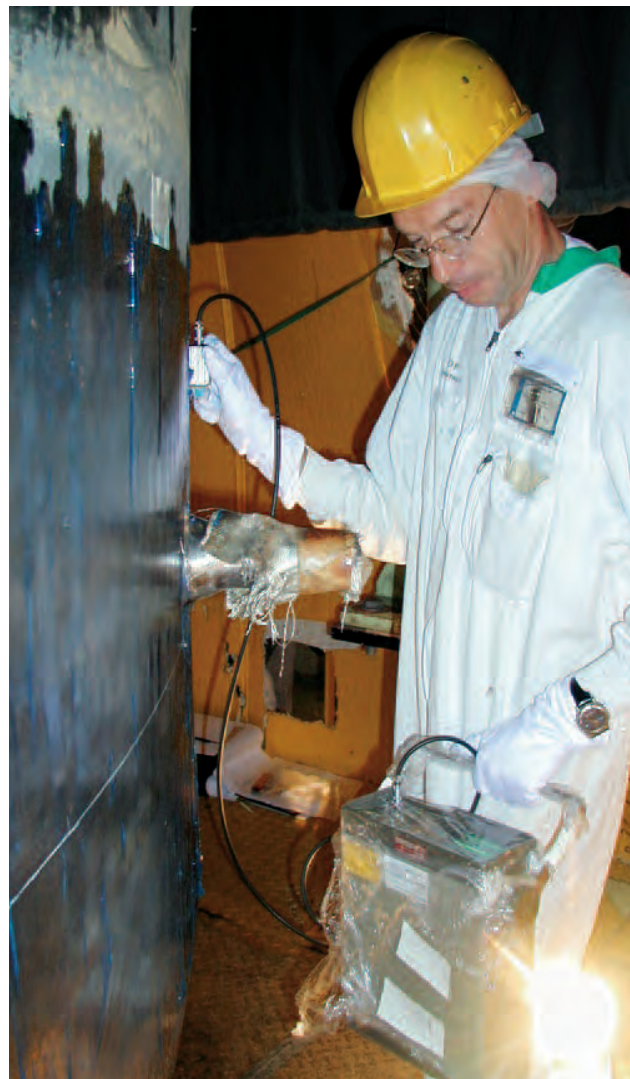
Ultrasonic inspection of a weld joint
